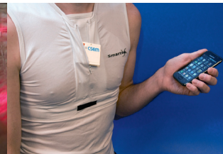
Real-time ECG device, for example in the context of obesity monitoring
