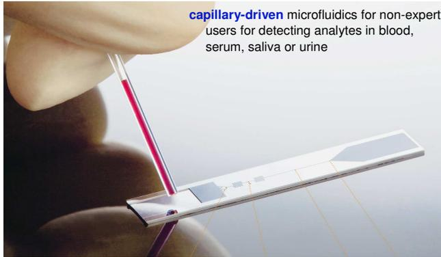
capillary-driven microfluidics for non-expert users for detecting analytes in blood, serum, saliva or urine
