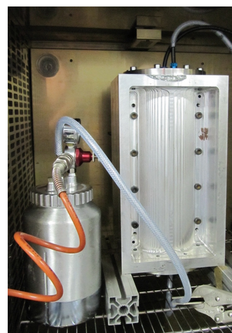
Resin Transfer Molding : Fabric impregnation with epoxy resin
