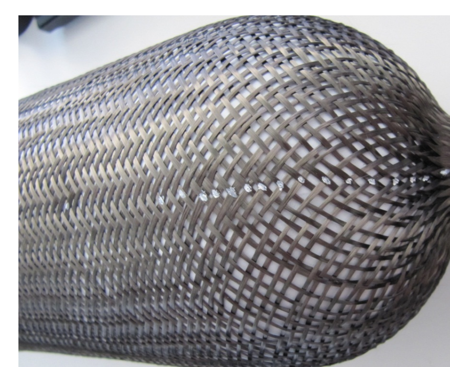
Carbon braid laminated over vessel shape
