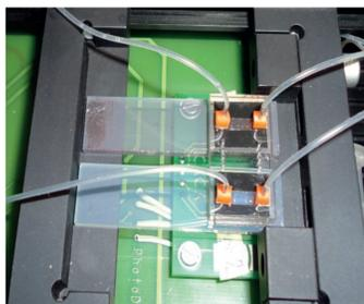
A microfluidics system consisting of two parallel channels has been built. One of the channels is used as a reference to compensate light drift and other artifacts by a differential measurement.
