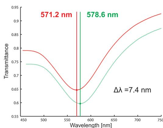
Peak shift of a single strand DNA layer: 7.24 nm with a dispersion of 1.65 nm over 11 samples.
