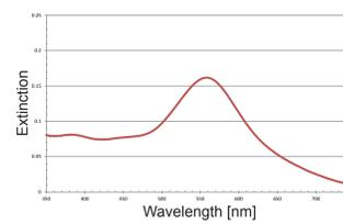
Extinction spectrum of a sample after evaporation and subsequent annealing.
