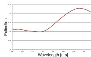
Extinction spectrum of a sample after gold evaporation.
