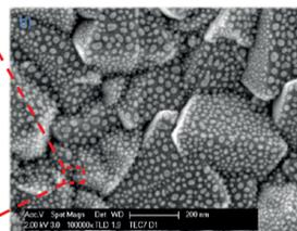
5 nm gold layer evaporated on a FTO glass substrate after mild thermal annealing.
