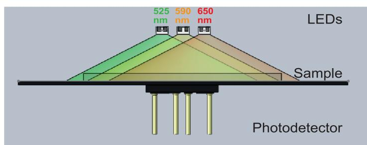
We developed a device based on low-cost off-the-shelf components, namely, electronically-driven power LEDs and photodetectors, and developed a novel data analysis approach that extracts the peak position of the LSPR spectrum from the measurements performed with a set of three LEDs.
