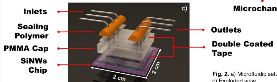
Fig. 2. a) Microfluidic setup. b) Top view; c) Exploded view.
