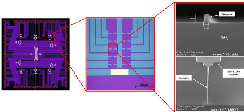
Fig. 1. Optical and SEM pictures of SiNW sensor devices. SEM pictures courtesy of CEA-LETI (Grenoble, France)
