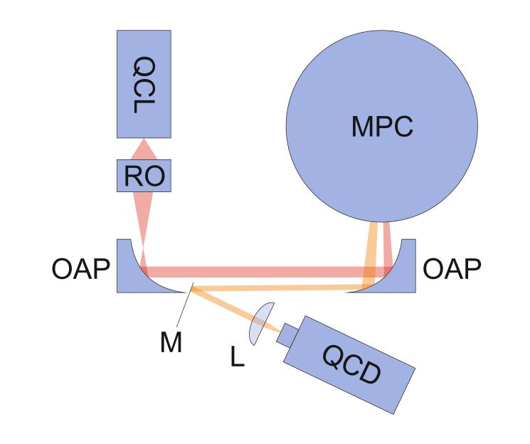
The laser beam is generated by a quantum cascade laser (QCL). A reflective objective (RO) and two off-axis parabolic mirrors (OAP) are used to shape the laser beam. The multipass cell (MPC) contains the sample gas. The collimated output beam is guided by a mirror (M) and focalized by a lens (L) onto a quantum cascade detector (QCD).
