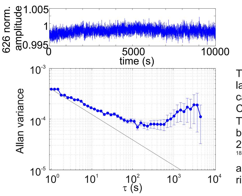
The combination of a quantum cascade laser, the toroidal gas cell, and the quantum cascade detector allows for high accuracy  $CO_2$  isotope composition measurements. The concentration of a single isotope can be measured with 0.07 ‰ accuracy after 200 s averaging (see on the left). The <sup>18</sup>O/<sup>16</sup>O ratio is determined with 0.1 ‰ accuracy after 600 s averaging time (on the right).
