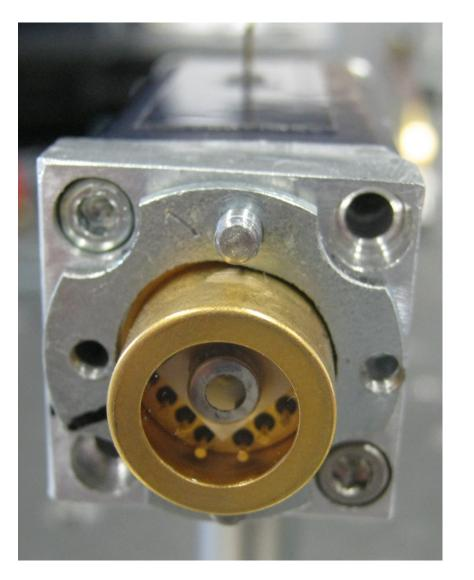
A quantum cascade detector is a spectrally narrow photon detector designed especially for mid-infrared light detection. The small spectral bandwidth allows for measurements with a very low background signal. Therefore, we obtain an outstanding signal-to-noise ratio in our setup.
