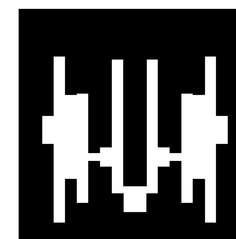
Meandered slot antenna optimized for Z_{CHIP} = 15 - j250 \Omega at 2.45 GHz (20 mm x 20 mm)
