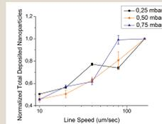
Total deposited particles per time in dependence of line speed.
