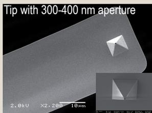
SEM image of FluidFM cantilever and pyramidal tip with aperture at the apex.
