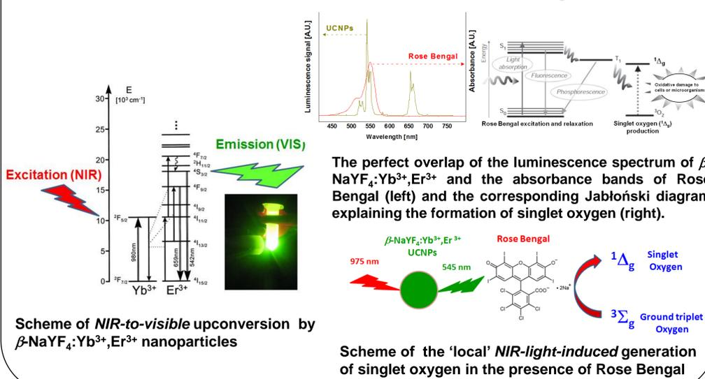
The perfect overlap of the luminescence spectrum of  $\beta$ -NaYF<sub>4</sub>:Yb<sup>3+</sup>,Er<sup>3+</sup> and the absorbance bands of Rose Bengal (left) and the corresponding Jablonski diagram explaining the formation of singlet oxygen (right).
