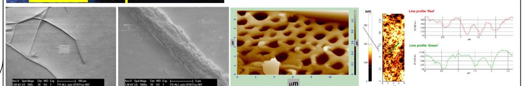
SEM and AFM images point to a very high porosity of the 'as produced' E-spun PS fibers loaded with UCNP and SPIONs, which is an asset in photocatalytic processes.
