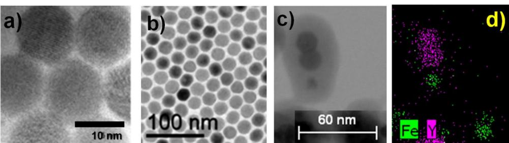
TEM micrographs showing the encapsulation of UCNP and SPIONs within silica shell (NaYF<sub>4</sub> &  $\gamma$ -Fe<sub>2</sub>O<sub>3</sub> @ SiO<sub>2</sub>): (a) individual custom-synthesized SPIONs, (b) individual commercial 30 nm spherical UCNP, (c) one SPION and two UCNP encapsulated in SiO<sub>2</sub>, and (d) EDX micrograph showing the elemental analysis of the nano-construct shown in (c).
