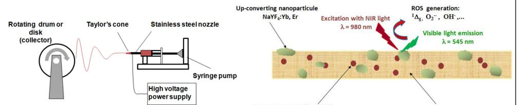
Schematic representations of: the custom-built E-spinning apparatus (left) and a multifunctional **magnetic**, **photoluminescent** and **photocatalytic** PS fiber loaded with SPIONs and UCNP, also doped with selected sensitizers of singlet oxygen, such as Rose Bengal or fullerene, C<sub>60</sub> (right).
