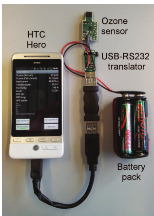
Low-cost ozone sensor connected to a HTC Hero
