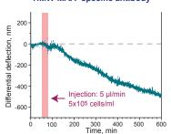
Sensor cantilever: antibody Mel-14 (HMW-MAA-specific) Reference cantilever: antibody 12CA5 (non-specific)
