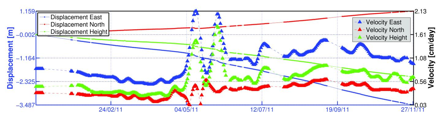
DI57, moving GPS station in Dirru rock glacier: relative position change (small markers) and estimated velocity (large markers). Blue, red, and green colors represent east, north and vertical components, respectively.
