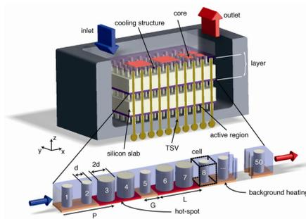
a) Chip stack with representative geometry modeled
