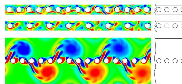
c) Laterally and longitudinally confined row of pins -> collaborative effect of multiple pins
