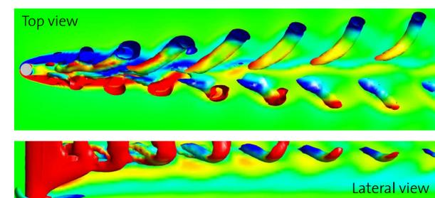
e) Vertically confined pin -> 3D vortical structures & endwall effect
