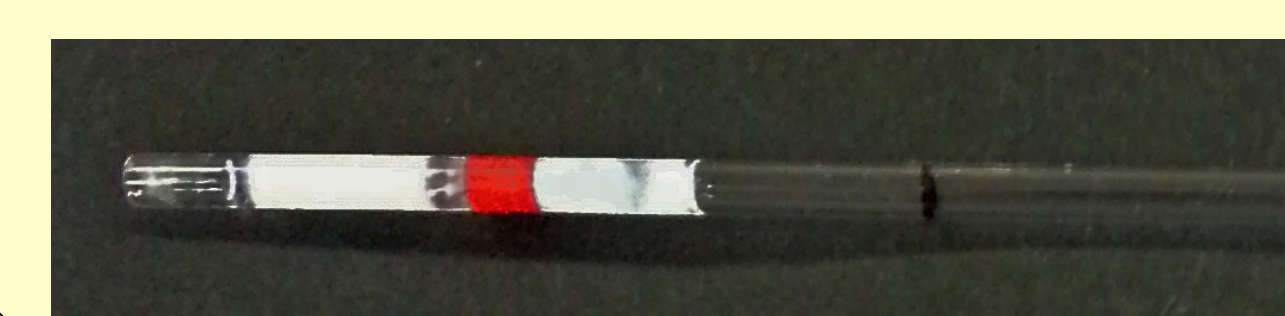
Figure 6: Tip of a capillary plugged by a porous monolith of polymer (poly-BuMA and EDMA) for cell retention.
