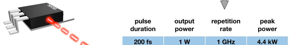
compact, low cost laser with high peak power for frequency comb generation
