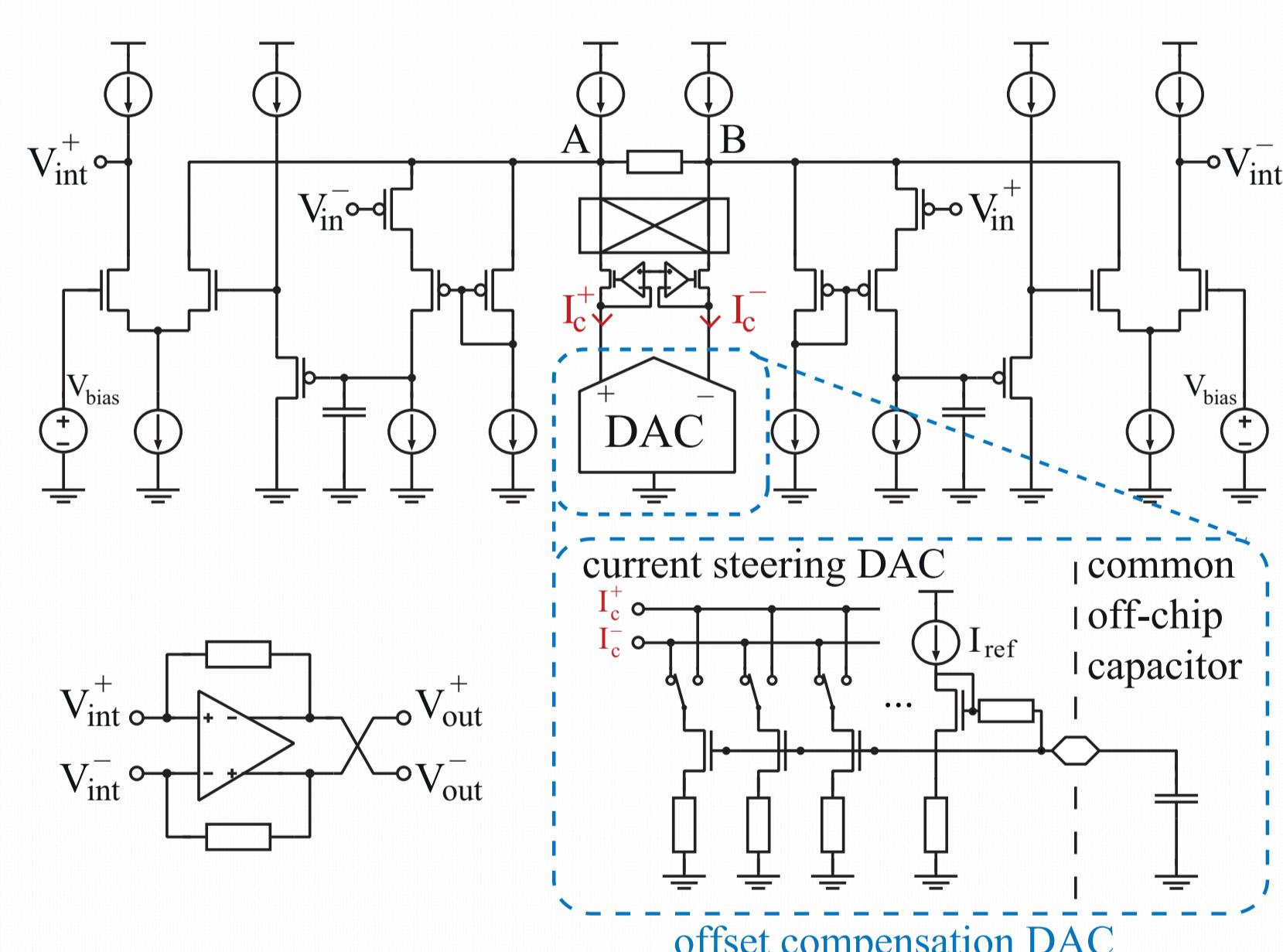
Fig. 3: Current balancing instrumentation amplifier (IA).
