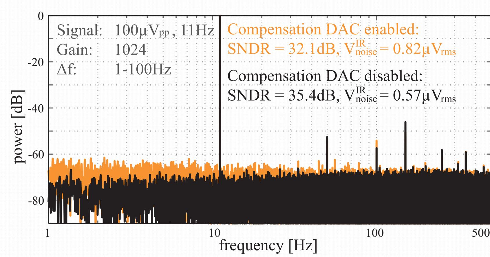
Fig. 5: Measured output spectrum of an electrode channel for an applied  $100\mu\text{V}_{\text{pp}}$  sinusoidal test signal with compensation DAC enabled (orange) and disabled (black).
