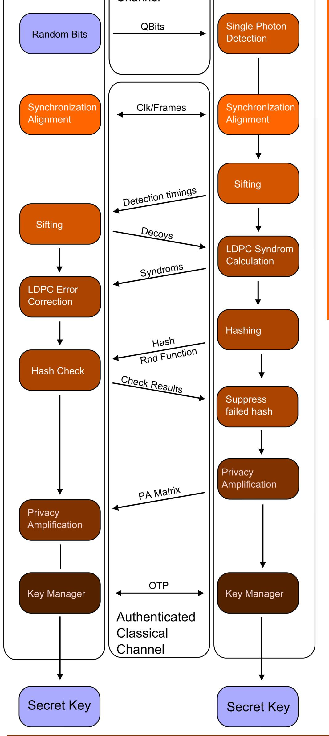
Both machines are completely synchronous, Bob recovers Alice's clock on the classical channel and forwards it to a jitter cleaner.
