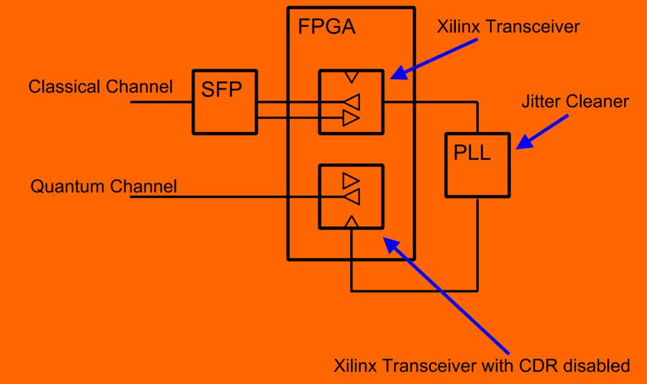
Specific frames are used to align the quantum channel with respect to the classical channel Data from the Quantum channel is sampled with a transceiver (Clock recovery disabled) synchronous with the emission
