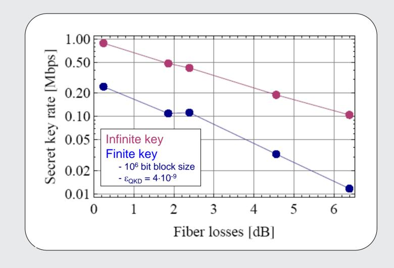
• Up to 890 kbps for short distances (250 kbps with finite key security) •More than 100 kbps over 20 km (12 kbps with finite key security) •Low QBER down to 1.7 %
