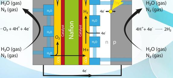
The solar cell will be fabricated using earth abundant materials (mainly silicon) and designed to provide the voltage to break the water molecules.
