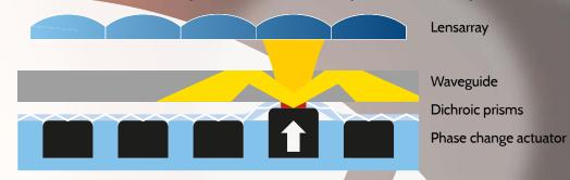
The self-adaptive mechanism uses the infrared light in the sunlight to create a local coupling feature by thermally expanding paraffin wax. Using a dichroic prism array in a flexible membrane visible light is reflected and coupled into the waveguide on contact between the membrane and the waveguide.
