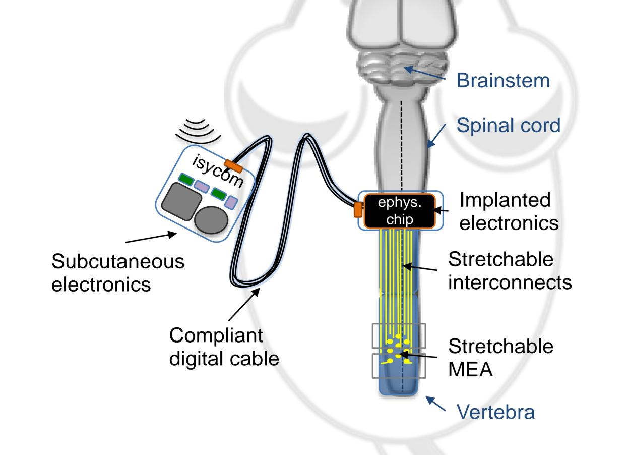
Schematic representation of the integrated spinal neuroprosthesis. The soft neural implant hosts ultra-compliant microelectrodes interfaced with miniaturised and power-efficient electronic circuitry linked to the digital and telemetry subcutaneous electronics board.
