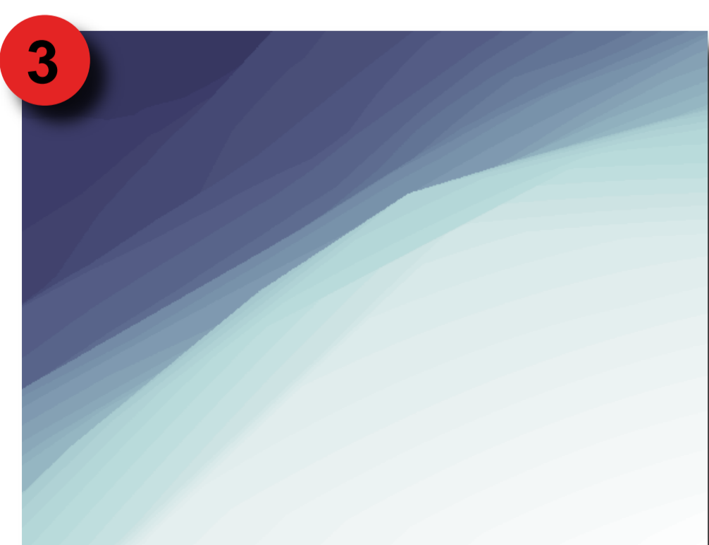
Z-buffer (image depth) computed using a 25m DTM (swisstopo) - bright areas are close to the camera
