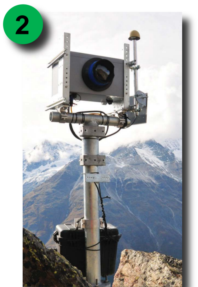
High-Resolution optical camera (12MP sensor with wide field lens) inside a robust weather proof mount and housing. A GPS antenna is mounted for position stability observation.
