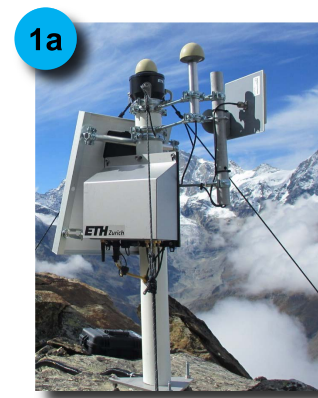
High-Resolution optical camera (12MP sensor with wide field lens) inside a robust weather proof mount and housing. A GPS antenna is mounted for position stability observation.
