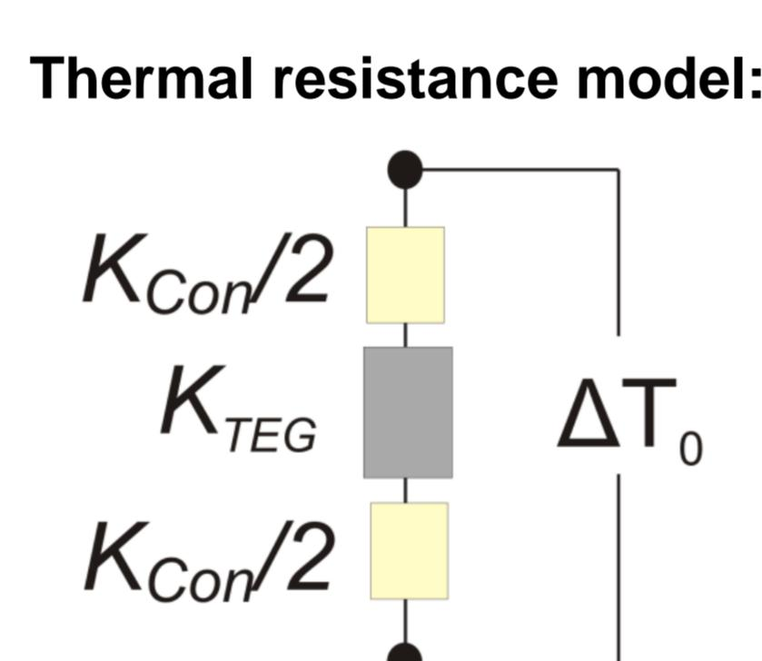
$$P_{TEG} = \frac{(m\alpha)^2}{4R_{El}} \cdot \left( \frac{K_{TEG}}{K_{TEG} + K_{Con}} \right)^2 \Delta T_0^2$$
