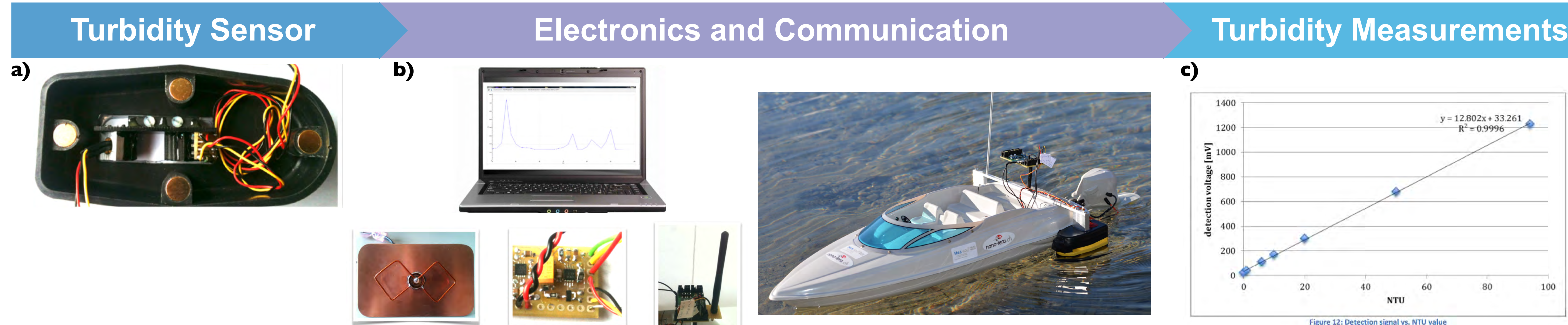
Figure 1. a) Optical image of the turbidity sensor that is controlled remotely by b) a circuit reader and a custom-built antenna on-board a remote control boat. c) Recorded signal as a function of different nephelometric turbidity unit (NTU) samples.
