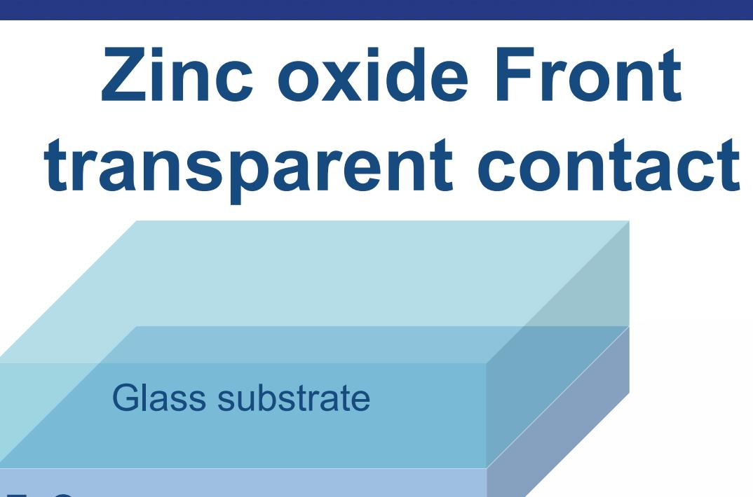
ZnO on glass substrate by low pressure chemical vapor deposition (LPCVD)
