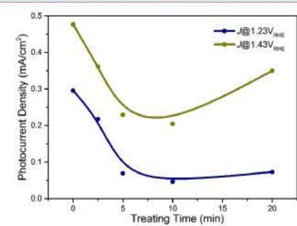
Photocurrent density reduced as expected and affected by treating time
