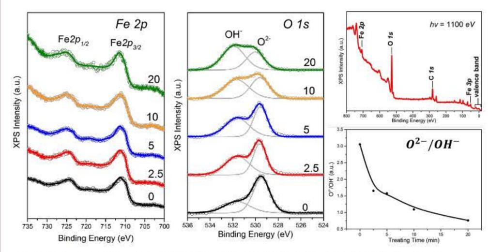
Hematite samples were prepared by dip coating methods and post treated with O2 plasma
