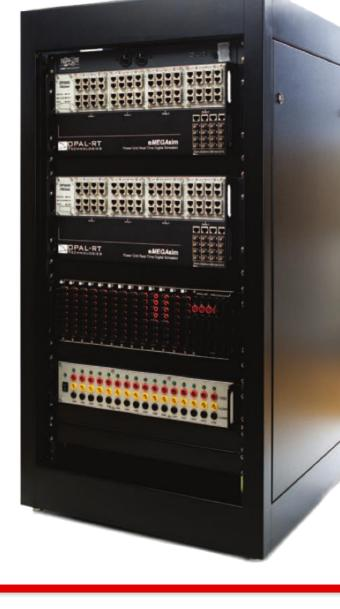
The algorithms that require the network to be in particular and non-desirable conditions (fault location, GPS attacks, etc.) are firstly tested by using a real-time digital simulator (RTDS). It allows the simulation of the network in any condition generating scaled analog output of the physical phenomena in real-time. PMU prototypes and all the chain described above can then be physically connected to the RTDS and tested.
