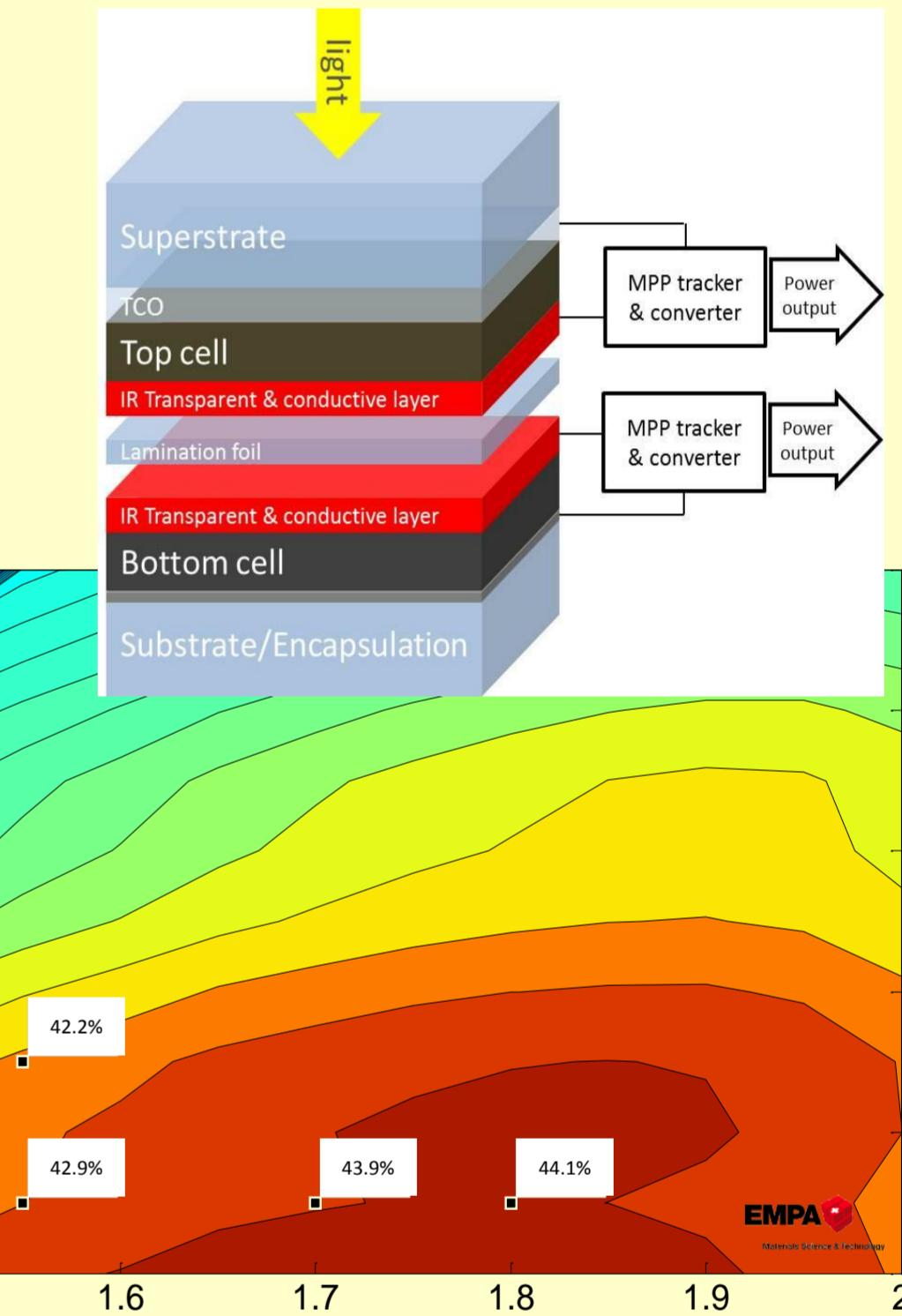
Detail balance analysis w/o optical losses in the transparent contacts
