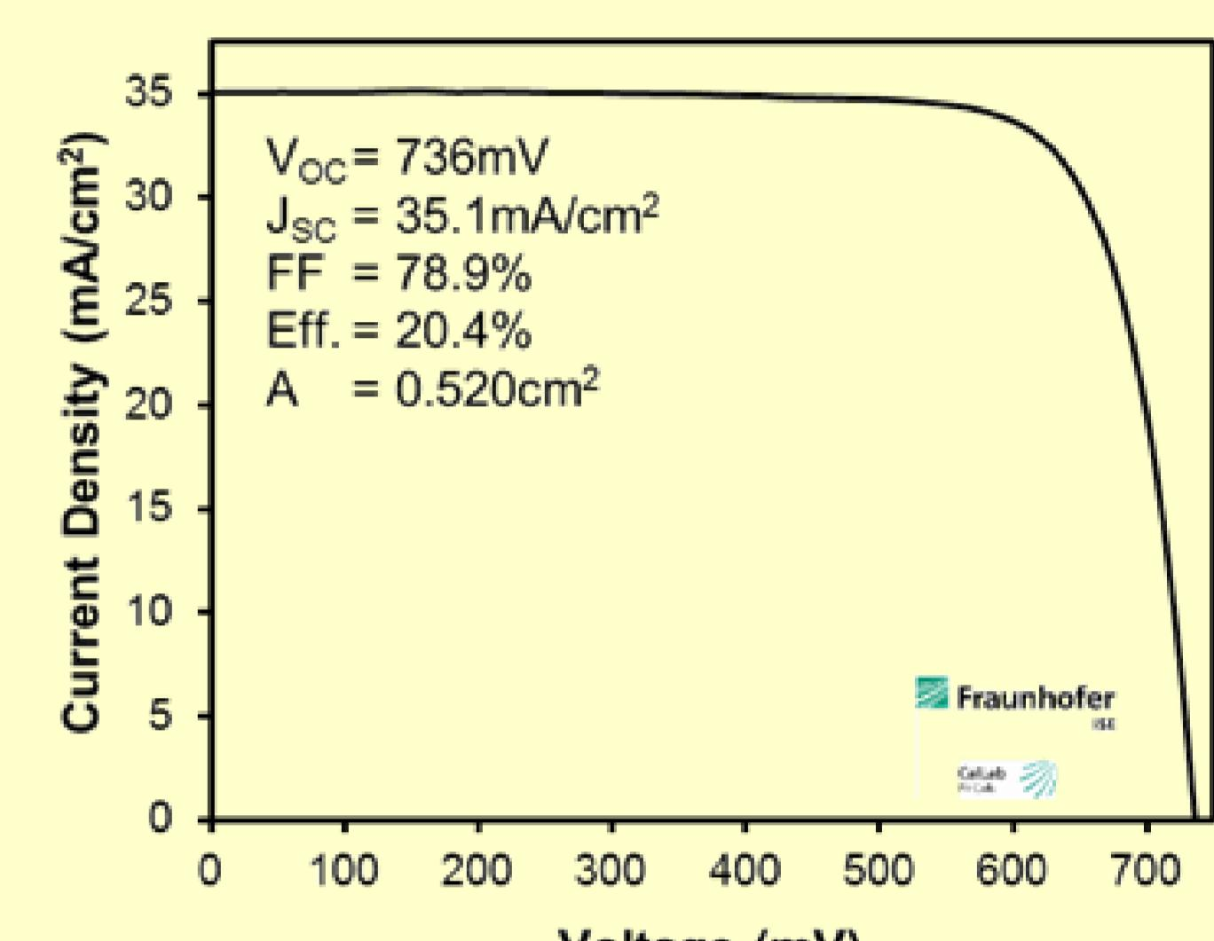
Flexible CIGS solar cell with 20.4% efficiency by low temperature deposition process
