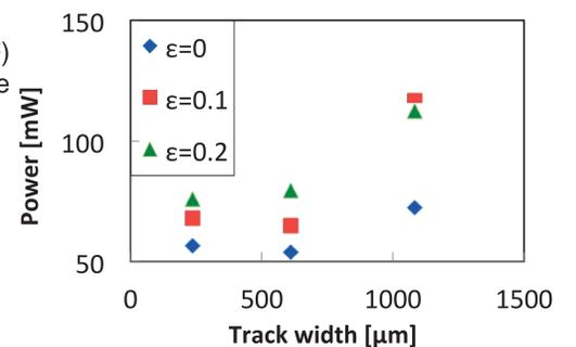
Dissipated power through stretchable gold tracks to reach  $\epsilon T_{max} = 60^\circ \text{C}$ , as a function of stretch.
