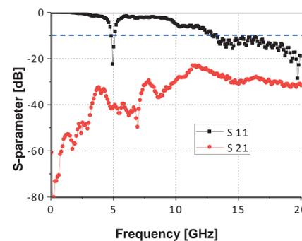
S-parameters for waveguide with top plane non-grounded
