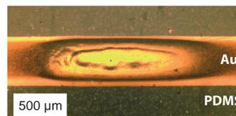
Damage induced by Joule heating
