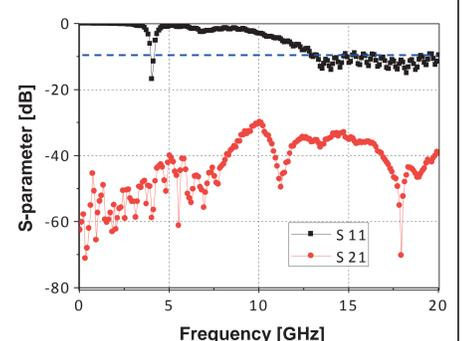
S-parameters for waveguide with top plane grounded
