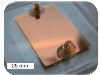
Conformable waveguide structure for propagation tests
