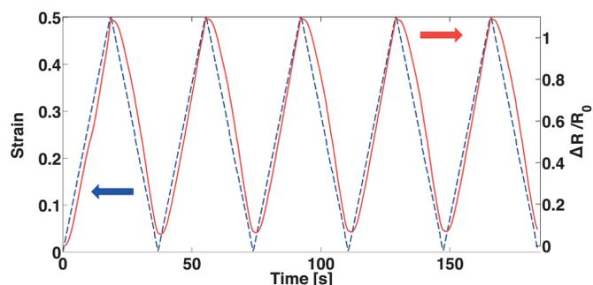
Resistance change of a 6x0.5 mm gold track on PDMS under large mechanical strain.
