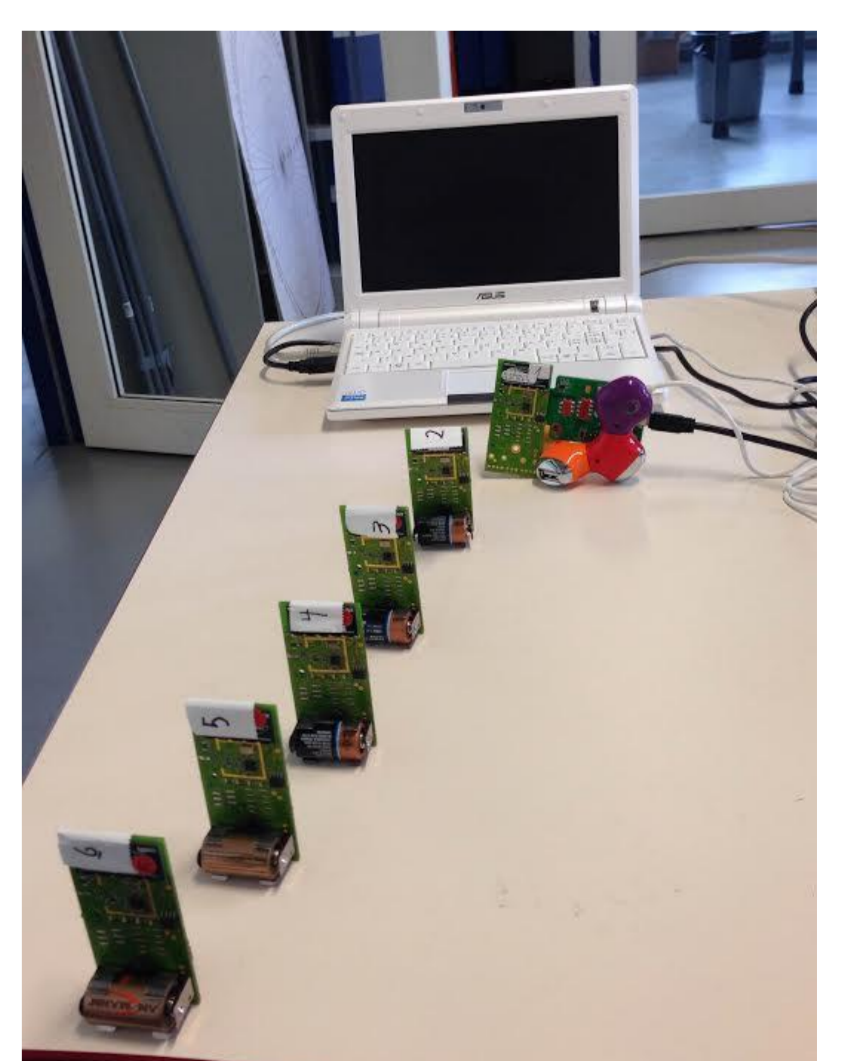
Figure 3. Test bed for understanding the end-to-end reliability
