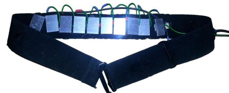
Thermal energy generators
