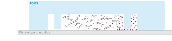
Filters prevent the cells to pass in the side channels thanks to their small height.
