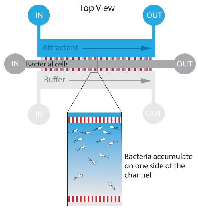
The chip is composed of three parallel channels connected by filters. By flowing attractant and buffer solutions in the side channels, we create a gradient in the middle channel, where cells are introduced.
