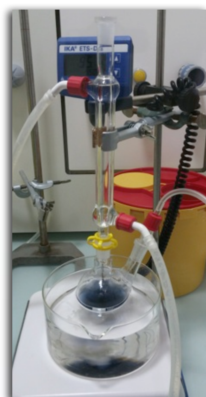
Figure 1. Synthesis of citrate-stabilized IrO x nanoparticles performed with a method described by Mallouk and co-workers. 3
