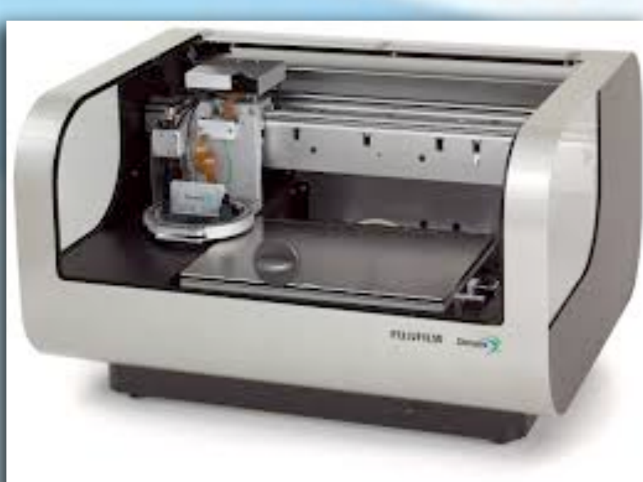
Figure 5. Printing of IrO x NP was performed using Dimatix inkjet printer DMP-2381. Ink was prepared by mixing of synthesized IrO x NP with Nafion and isopropanol.
