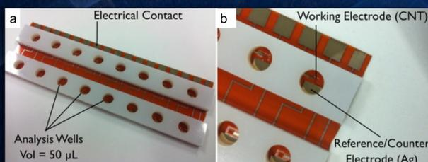
Picture 2: Inkjet printed microchip employed for the bioelectrochemical monitoring of Hg (II). The microchip contains 16 independent electrochemical sensors (a), each one (b) consisting of a two-electrode setup (working electrode CNT, counter/reference electrode Ag) and a well (50  $\mu$ L) made in Plexiglas.
