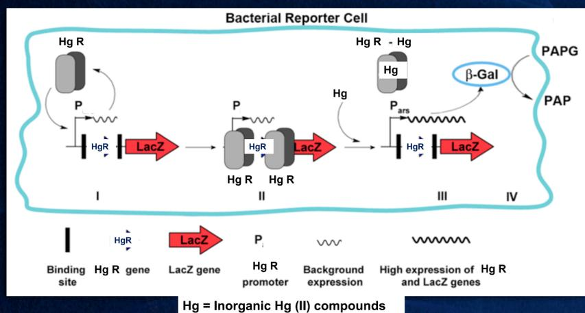
Figure 1. Detection mechanism of the Hg (II) bioreporter:
