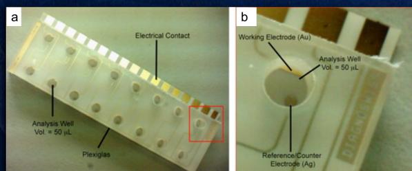
Picture 1: Diagnoswiss microchip employed for the bioelectrochemical monitoring of Hg (II). The microchip contains 16 independent electrochemical sensors (a), each one (b) consisting of a two-electrode setup (working electrode Au, counter/reference electrode Ag) and a well (50  $\mu$ L) made in Plexiglas.
