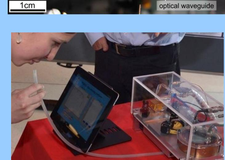
Laboratory based CO<sub>2</sub> isotope analyzer
