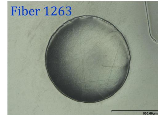
The fibers are extruded from a commercial block copolymer containing urethane and siloxane units. As a mono-component fiber without cladding, they are highly susceptible to lightoutcoupling as schematically pictured below. The fibers' diameters and mechanical properties vary with extruding temperature, cooling conditions and roll-off speed. Additionally, the chain length of the siloxane block has been varied. With longer chains, the pressure sensitivity increased dramatically.
