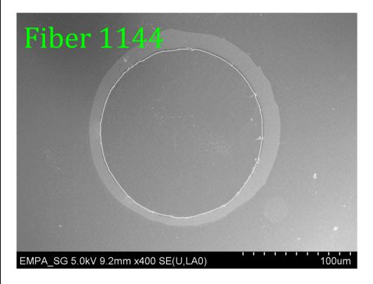
The fibers 1143 and 1144 are co-extruded at 300 and 400 m/min respectively, thus allowing for fast and continuous production. Both core and cladding are commercially available. The fluorinated polymer for the cladding makes the fiber highly resistant to environmental influences and allows for total light reflection inside the fibers' core.
