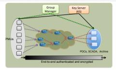
Secure end-to-end multi-cast communication
