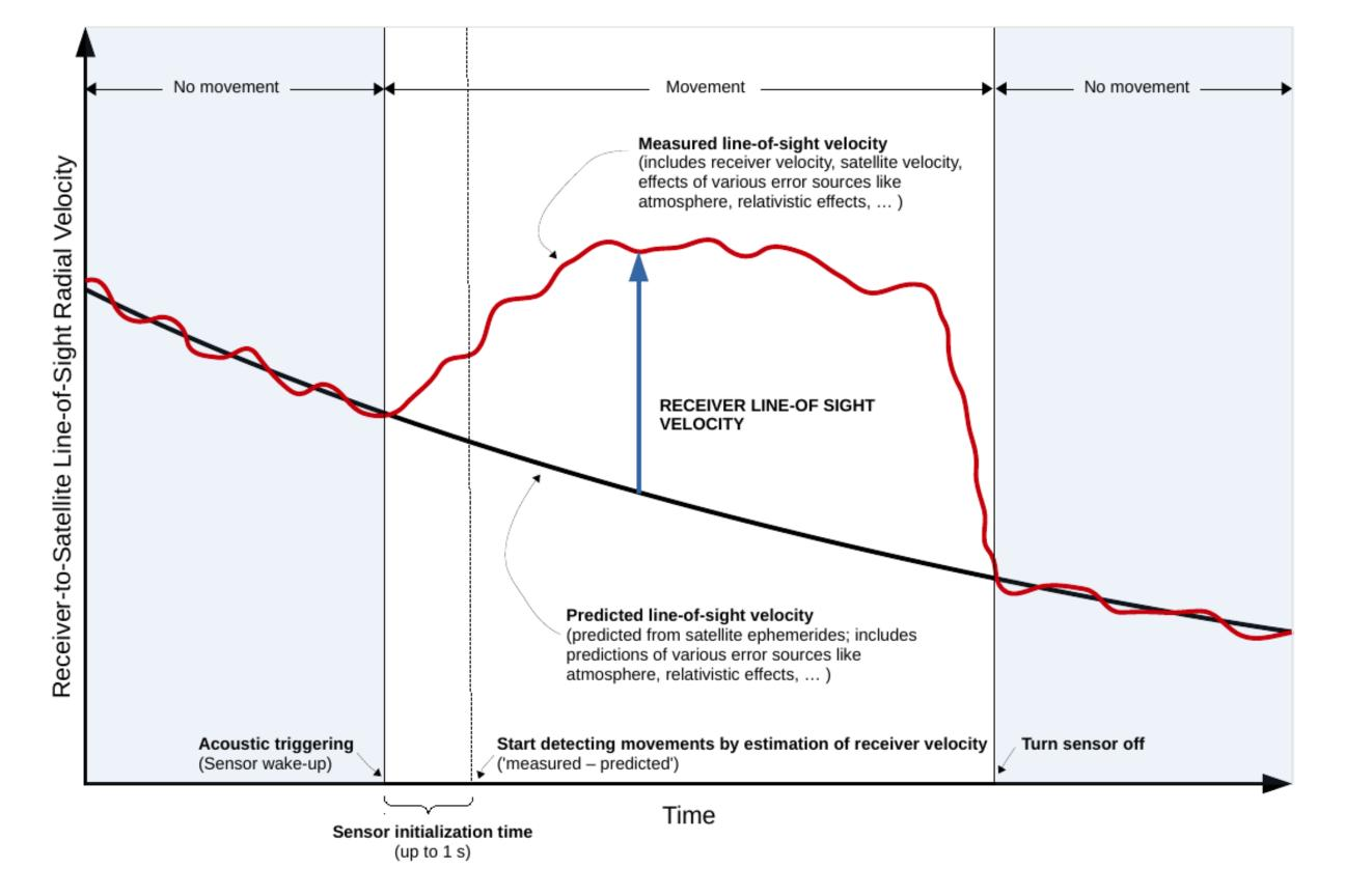
• Concept based on prediction of contributing effects (analytical and empirical models) to observation equation in the velocity domain
