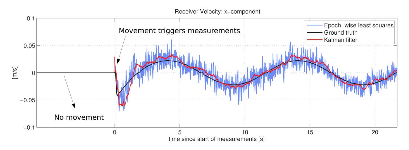
In this case study, small movements can be tracked with Doppler measurements of a high-grade GPS receiver
