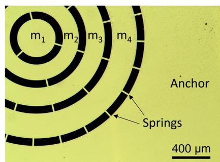
Optical microscope partial top view of N4.
