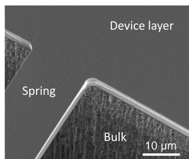
Tilted SEM image of a double clamped beam (spring).
