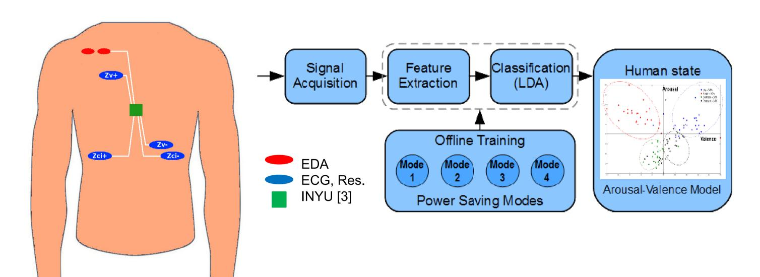
Optimal sensor placement to reduce artefacts.
