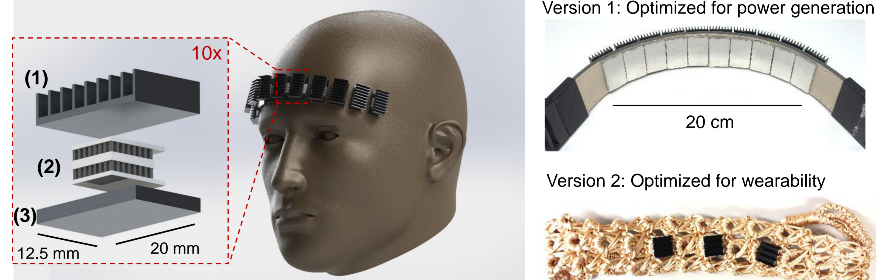
Fig 5: System overview (center), closeup of the harvester module (left) and prototypes (right). (1) Heat sink ( R_{th} = 20 \text{ K/W} ) to dissipate heat into the environment. (2) Stacked TEGs ( R_{MT}, R_{el} = 13.33 \Omega , R_{th} = 85 \text{ K/W} ) for power generation. (3) Hot interface (AI, A = 4 \text{ cm}^2 ) to increase effective harvesting area.
