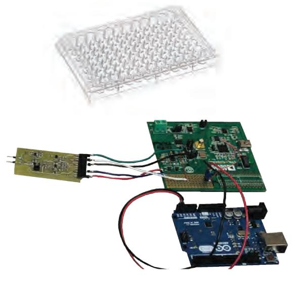
"Reference-chip" was a commercial 96-well plate with electrodes and external measurement unit supplied by the manufacturer. The device was not integrated or portable. "Envirochip" was a 96-well culture plate engineered by us, with embedded electrodes similar to the Reference-chip. Both chips were further manipulated: cables were directly attached to the wells, then connected with a portable external measurement unit. Image on top shows
