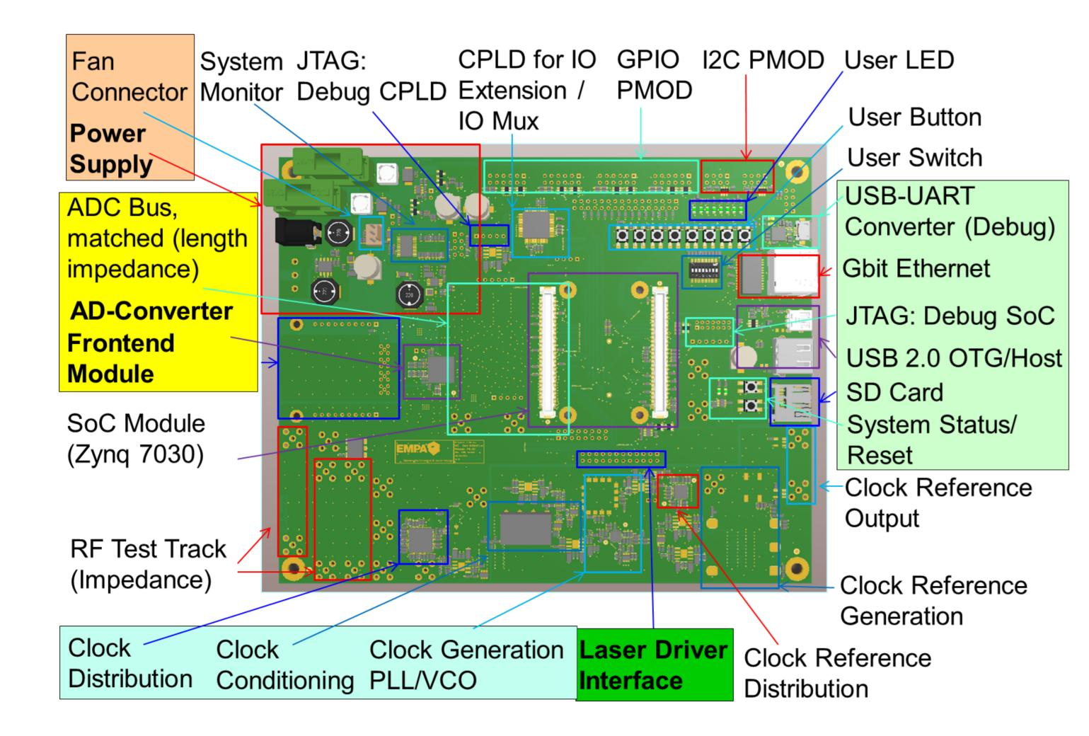
With the DAQ2 first gas cell absorption measurements were performed. The quasi-static QCL [1] driver (pulse length > 1  $\mu$ s) is triggered by the board producing a chirped laser pulse directed to a detector passing a CH<sub>4</sub> containing cell. The signal is digitized at 310 Ms/s and averaged without losses.
