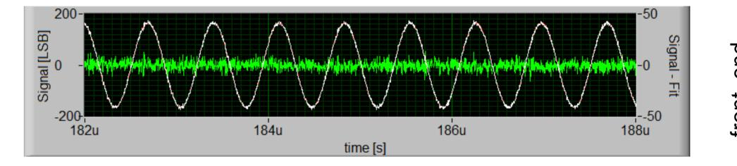
The analog front end can be exchanged to be adaptable to various needs. The new active front end has a flat frequency response compared to the simple balun front end. Cross talk for dual channel ADC is important. Up to 10 MHz cross talk is below -80 dB.
