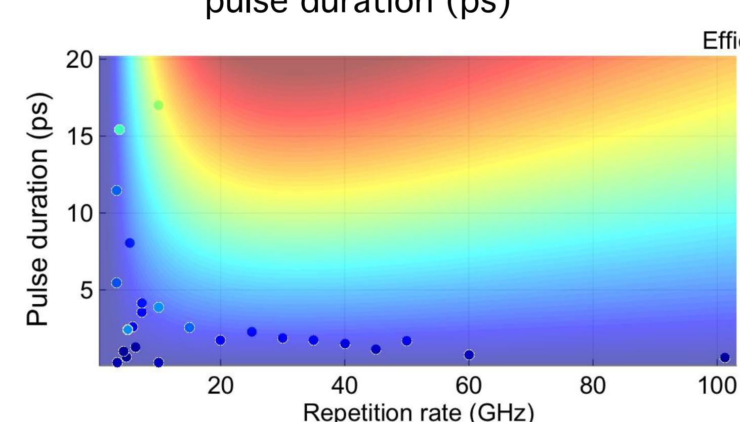
MIXSEL data points fitted to a model for efficiency simulation
