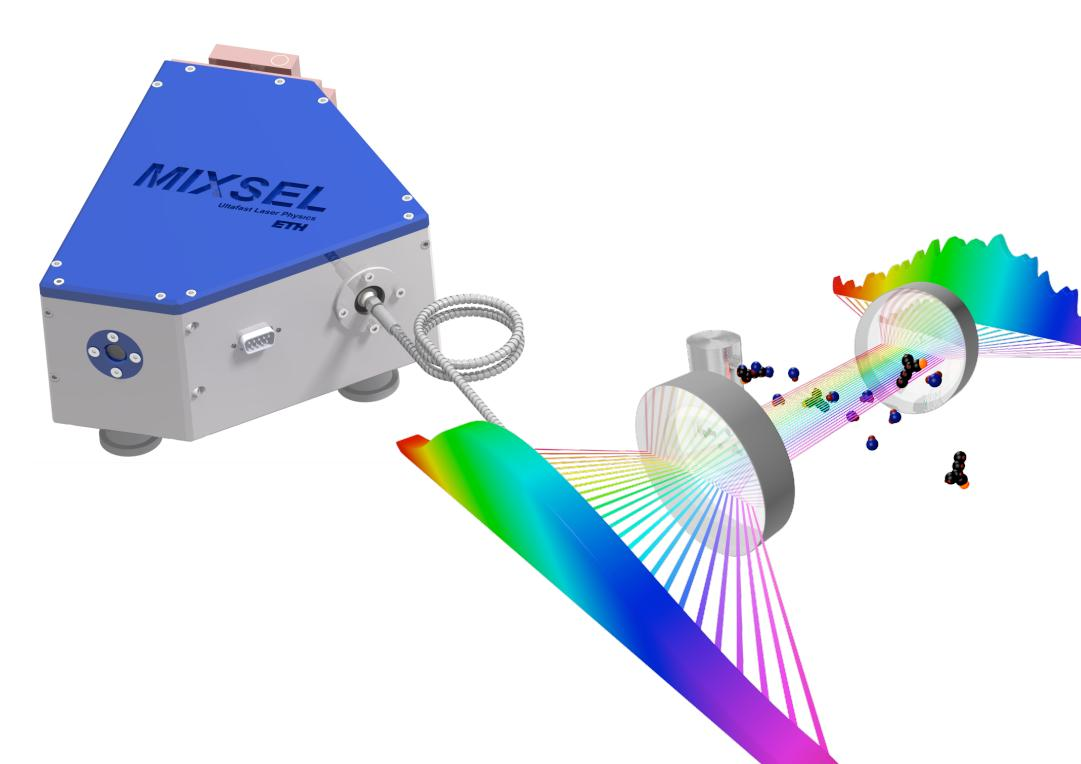
next steps: sub-200-fs pulses with > 1 kW peak power from a MIXSEL
