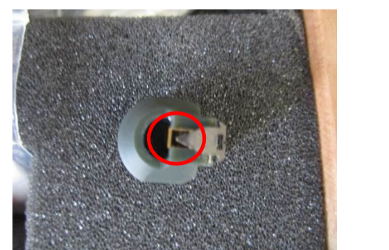
Fig. 2.6: Cantilever array holder. The gold colored part is the cantilever array (marked by a red circle).
