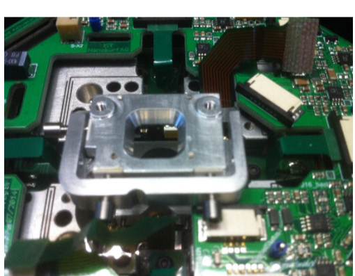
Fig. 2.3: The VCSELS' holder is inserted in the FlexAFM head to replace the production series laser unit. The optical path is chosen in such a way that the laser light falls onto the position sensitive detector (PSD).
