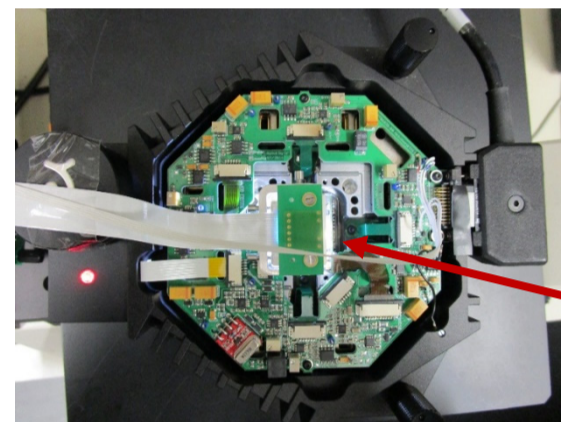
Fig. 2.4: Top view of the FlexAFM head with mounted VCSELS' holder and VCSELS.
