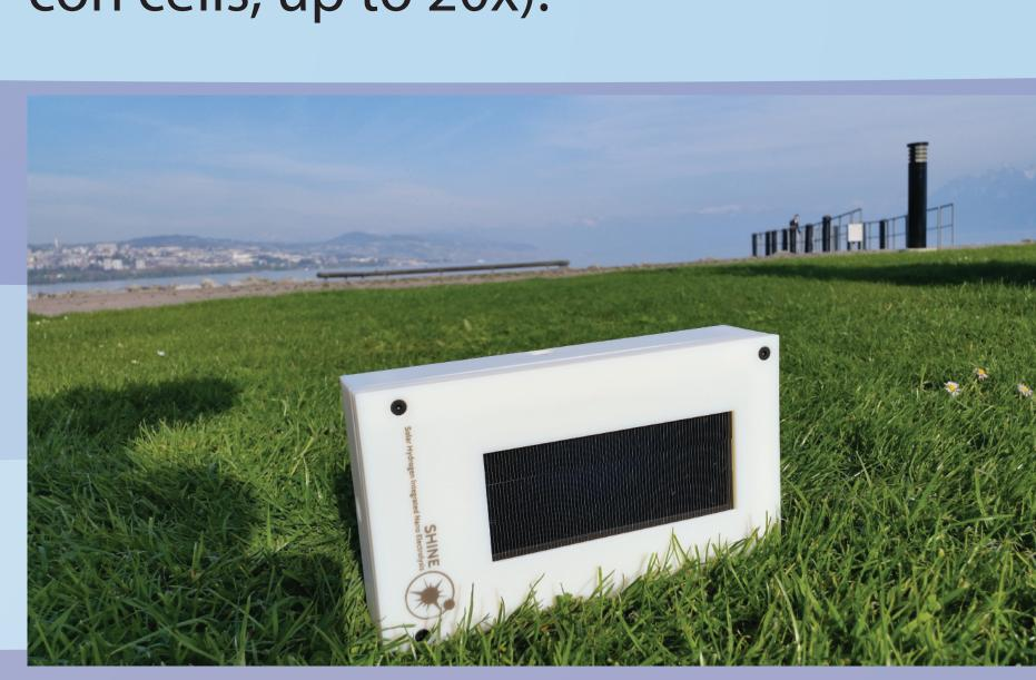
Based on a phase-change actuator, a scalable prototype was assembled. The device showed a concentration factor of 3.5x (16° acceptance angle)<sup>[5]</sup>.
