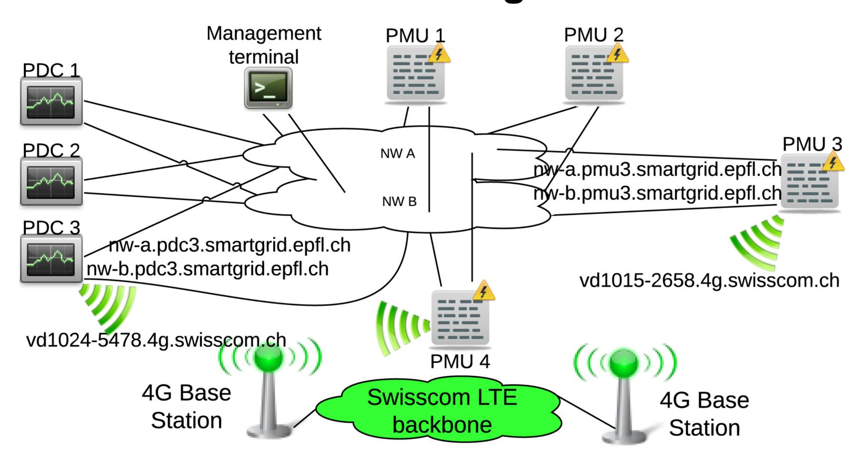
On the sender side (PMUs): packets are replicated and sent over fail-independent networks.
