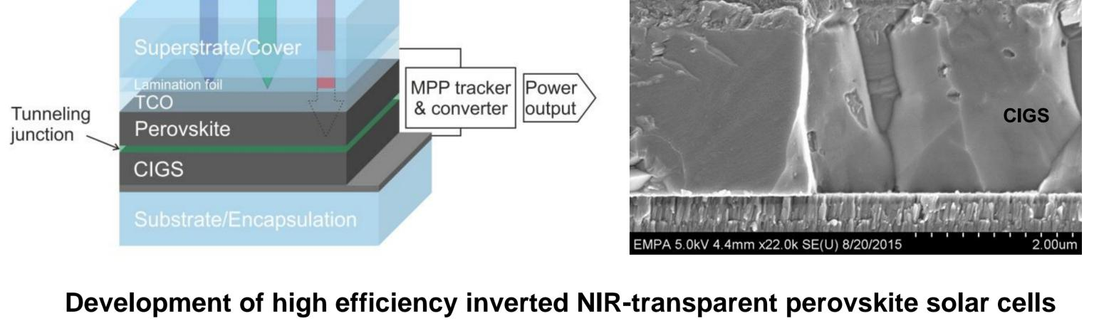
is critical for 2-terminal perovskite-CIGS tandem devices
