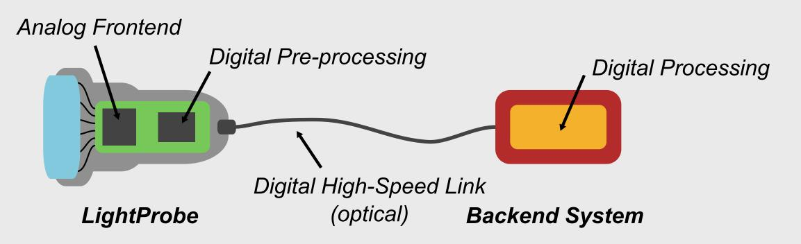
The analog frontend is moved into the transducer head. Pre-processed **digital samples** are sent over an **optical digital link** to a backend processing system. All ultrasound-specific hardware is concentrated in the transducer head (LightProbe), which can be connected to a **commodity processing platform** over a standardized interface.
