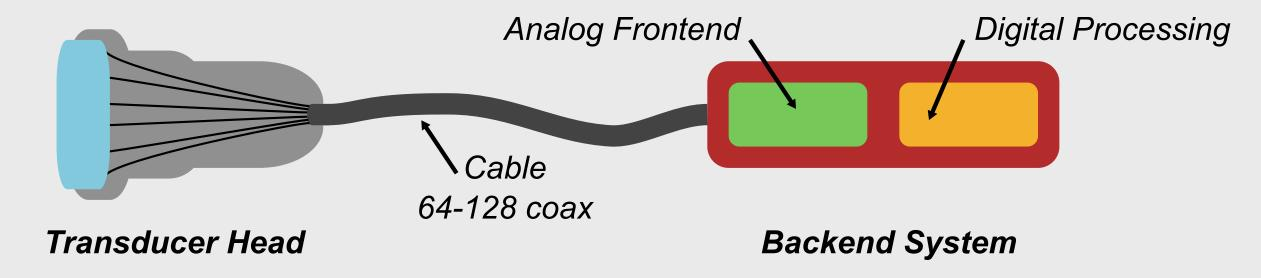
The transducer head is connected over an **expensive micro-coaxial cable harness** to the backend system.
