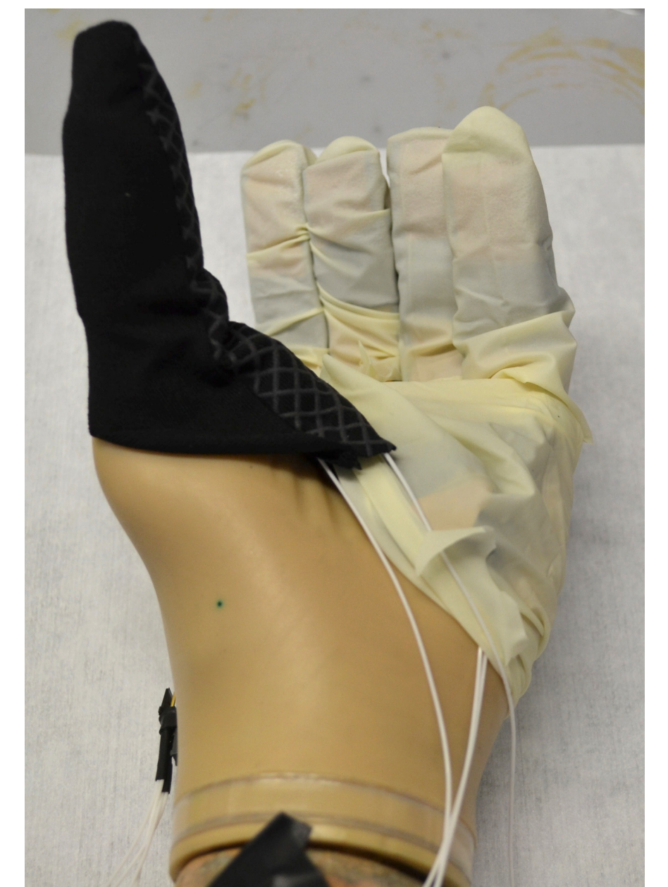
WiseSkin system integrated on the Ottobock Myohand Varyplus prosthetic hand
