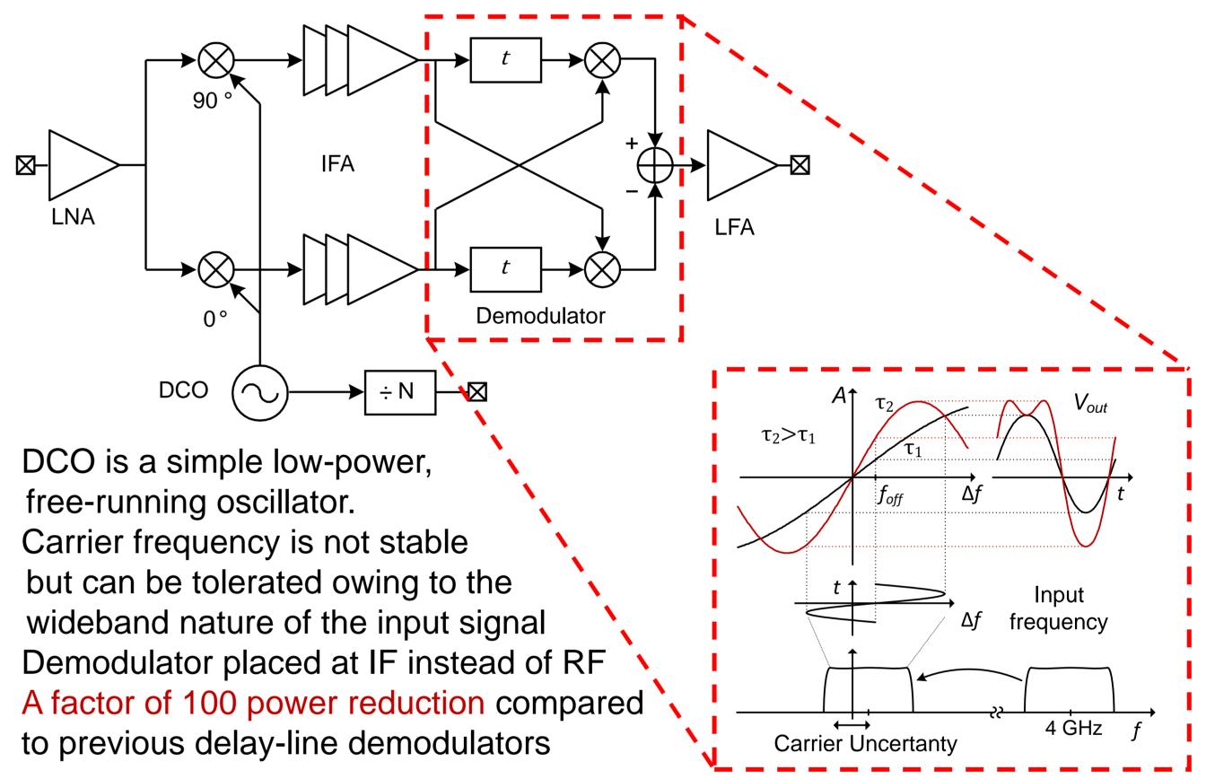
The aim of this work is development of an ultra-low power receiver that will be used for communication between the sensor nodes
